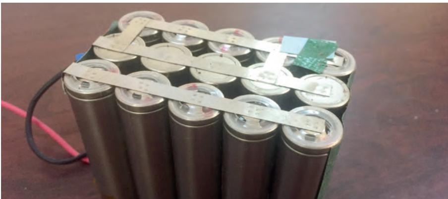
Typical arrangement of Li-ion cells for a battery pack used in SHS
